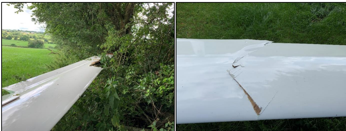
Photo No. 3 and No. 4: Damage to the left wing
