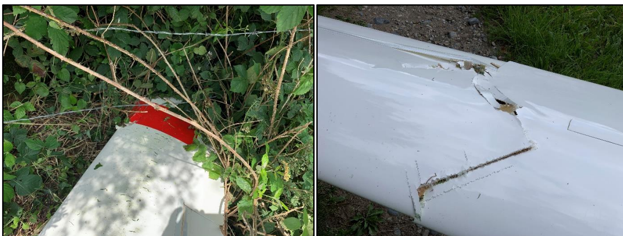
Photo No. 5 and No. 6: Damage to the right wing
